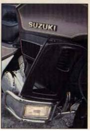
Vents in lowers use remote-controlled guillotine-style doors with infinite adjustability. Cornering light housings do double-duty as forward floorboards.
