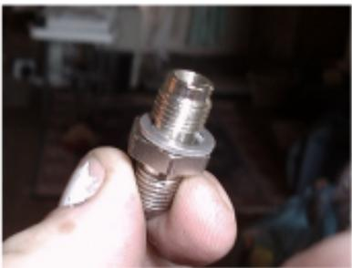
2) Wipe the area around the hole in the caliper clean, install a crush washer on the flat end of the new adapters (they are threaded into one end of the new lower lines), and thread the new adapters in place of the old. Tighten to 14.5-18 ft/lbs (9/16" size).
