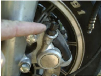
1) Disconnect the lower front lines from the calipers at the swivel joint and remove the swivel adapter from the caliper.
