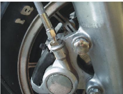
7) Thread the swivel nut on the lower end of the line onto the adapter fitting installed into the caliper on step 2. You can turn the line so that it's natural curve fits it's location. Tighten the swivel nuts on both ends of the line (7/16" wrench). Since they seal on a taper, they need to be good and snug but not overly tight.
