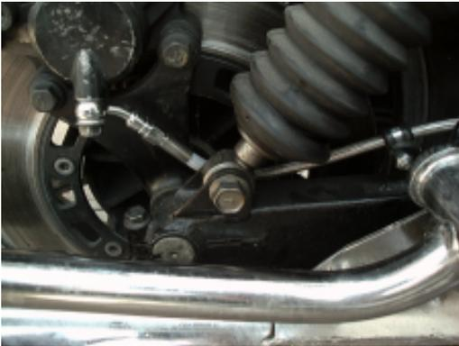
6) Move the Adel clamps to line up with the existing brackets and squeeze them shut around the line. Using the included self-locking nut and the original bolt, attach the rear clamp to the rear bracket. Using the included aluminum block, attach the front clamp with the original bolt.
