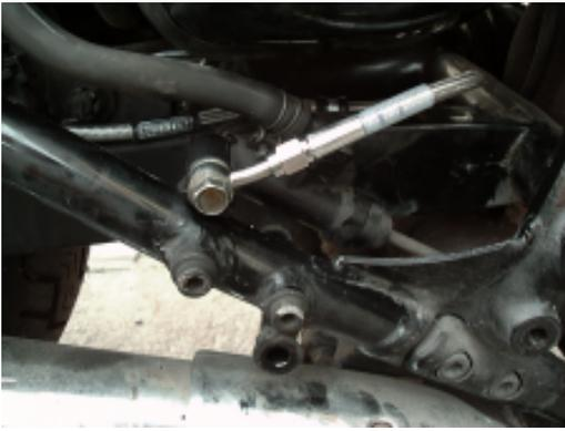
5) Connect the line at the caliper and master cylinder using new crush washers on both sides of each fitting and tighten the banjo bolts to 14.5-18 ft/lbs. Once the fittings are tight, go ahead and tighten the swivel nuts to the fittings with a 7/16" wrench. Since these connections seal on a taper, the nut doesn't need to be overly tight.
