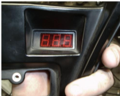
5) Slide the meter behind the leg of the left bracket installed in step 3 and attach it to that bracket with the remaining included screw and lock washer. Leave the screw a little loose. Attach the right bracket to the dash panel with the other blank-plate screw and just snug it.
