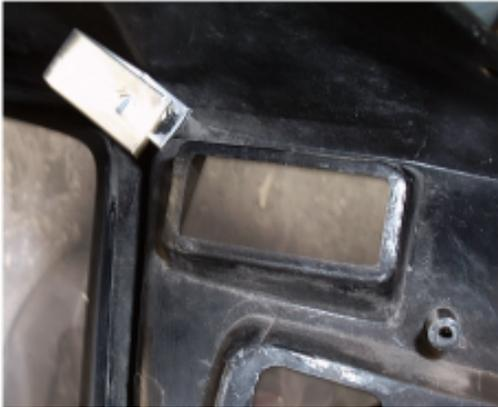
2) Remove the blank plastic cover over the left-hand opening. Save the screws, you will reuse them.
