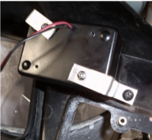
4) Attach the remaining bracket (legs bent in opposite directions to the back of the meter with one of the included screws to the right-lower hole drilled into the back of the meter. Use one of the included lock washers between the screwhead and the bracket. Leave the screw slightly loose.
